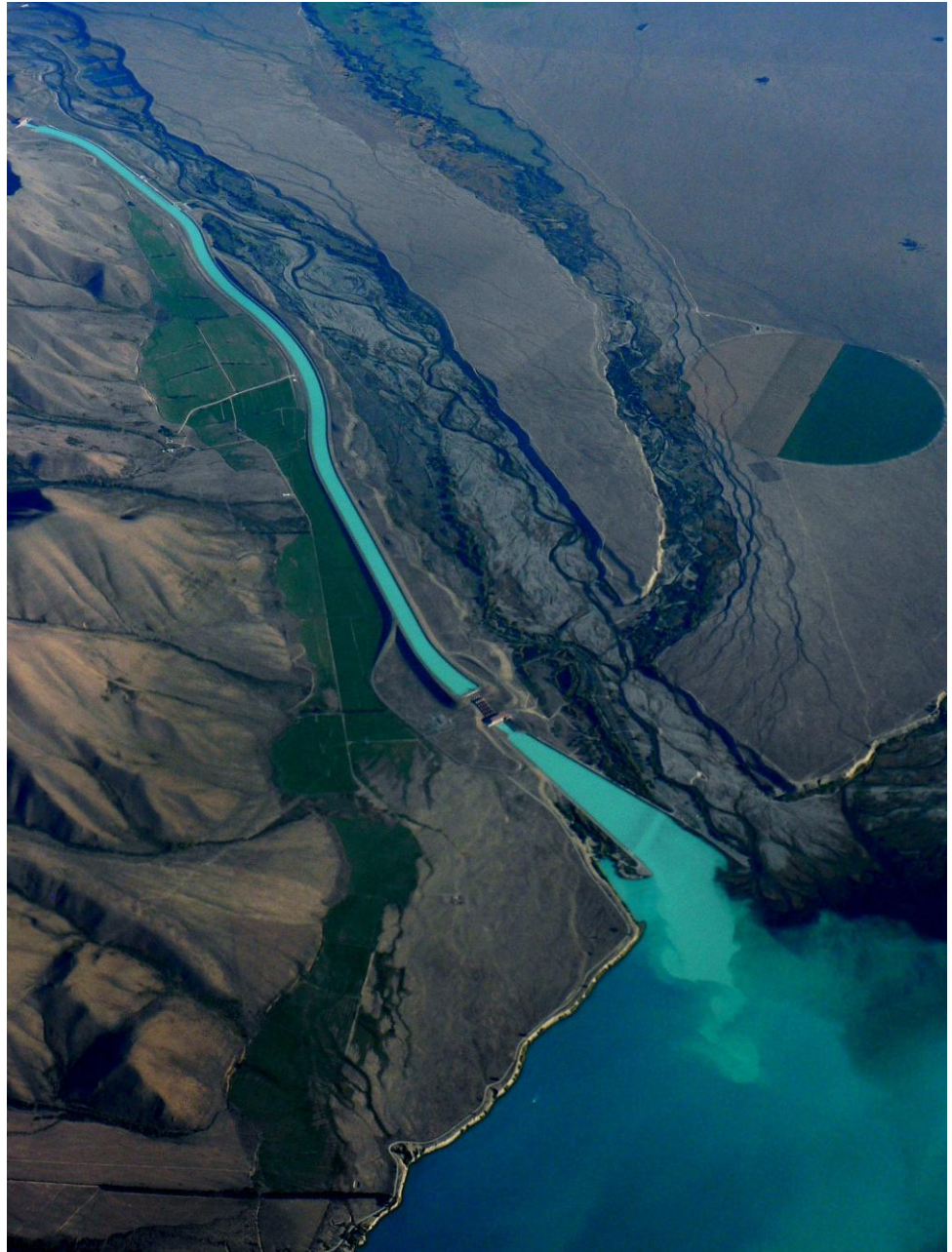
Plate 1. Distinct zonation of inflow waters from the Ohau C Canal, lower Ohau River and Tekapo / Pukaki River. The low mixing zone of the Tekapo / Pukaki River extends past the right of the photo.
