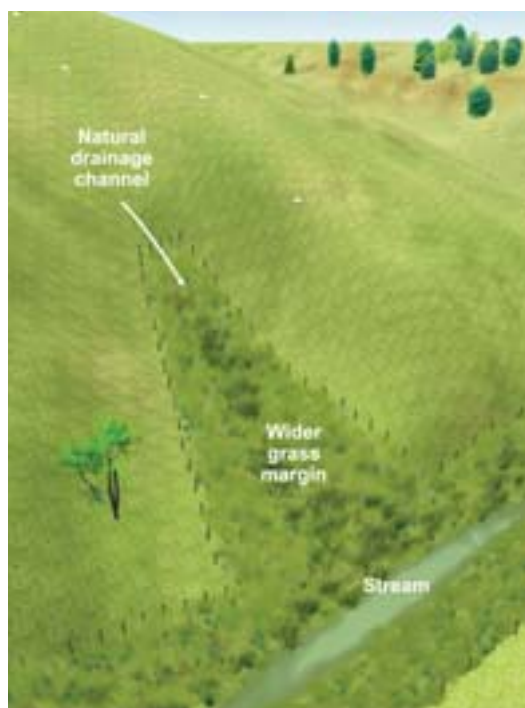
FIGURE 4 Using grass margins to filter channelled run-off from low points in paddock.
