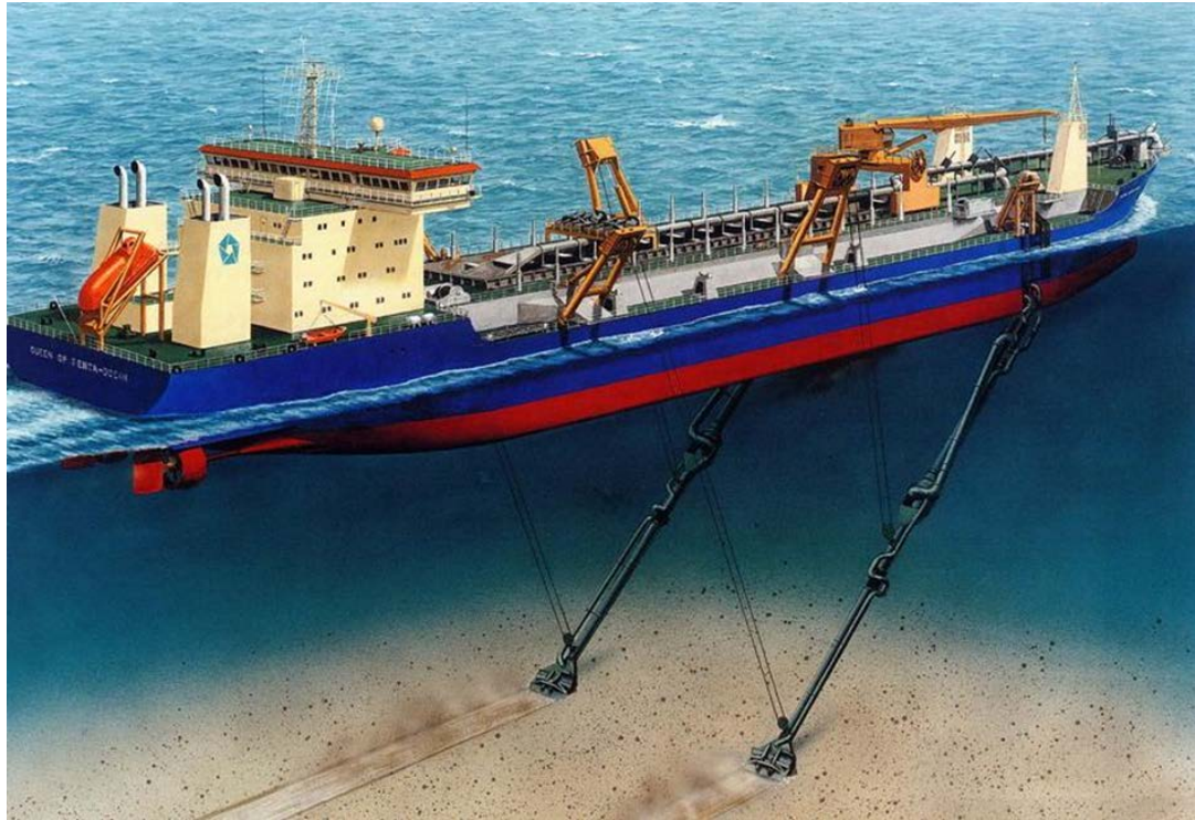
Figure 2: showing a trailer suction hopper dredger typical of that to be employed for the CDP
