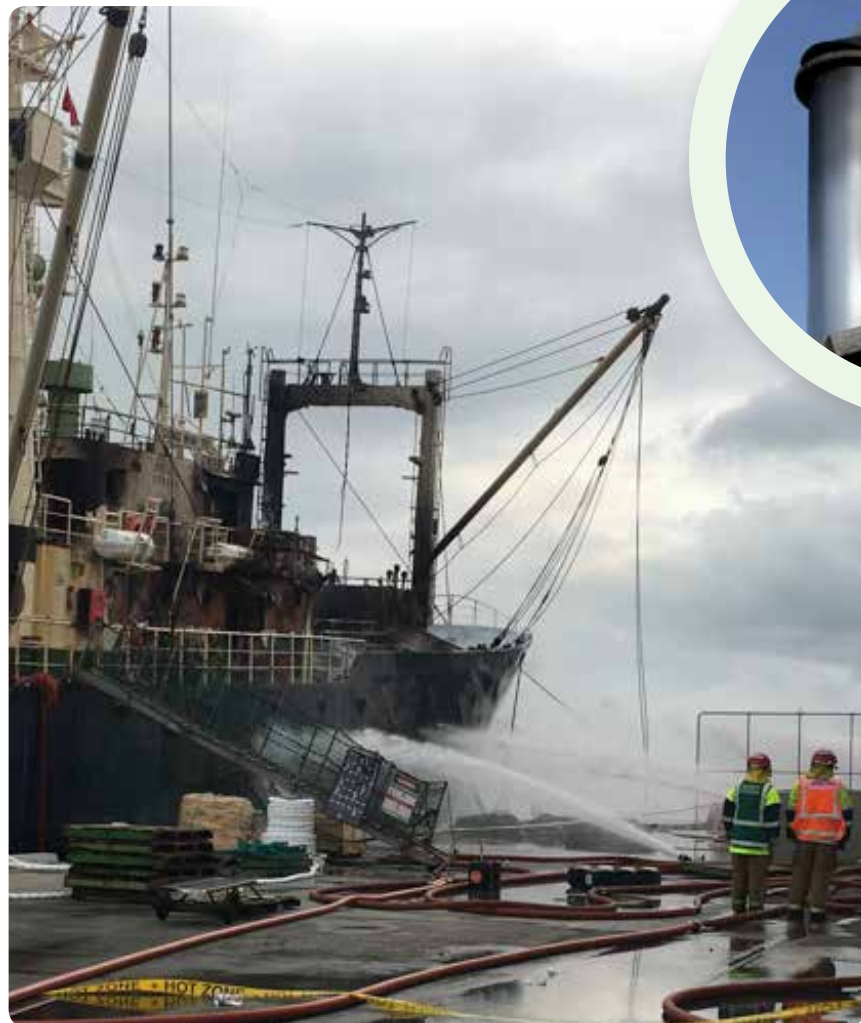
Water is being sprayed on the hull of the vessel to cool down the outside and stop fire from spreading.
