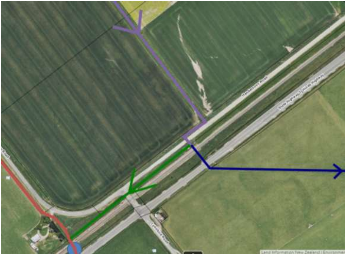
Map 5B: Rerouted drains to the east. The purple line is the field drain, the dark blue is where the water used to go, the green line is the rerouted watercourse.
