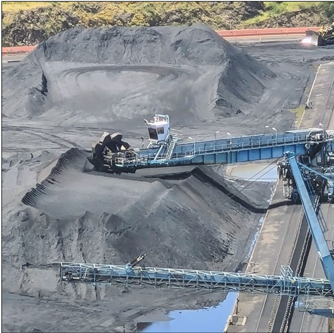
Figure 2.5: The bucket wheel reclaimer taking coal off a stockpile which is then conveyed to the north-side of the coal stockyard and then conveyed to a vessel for loading. Source: Tonkin & Taylor
