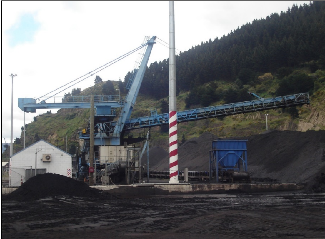
Figure 2.4: Stockpiles being formed using the gantry stacker. Source: LPC
