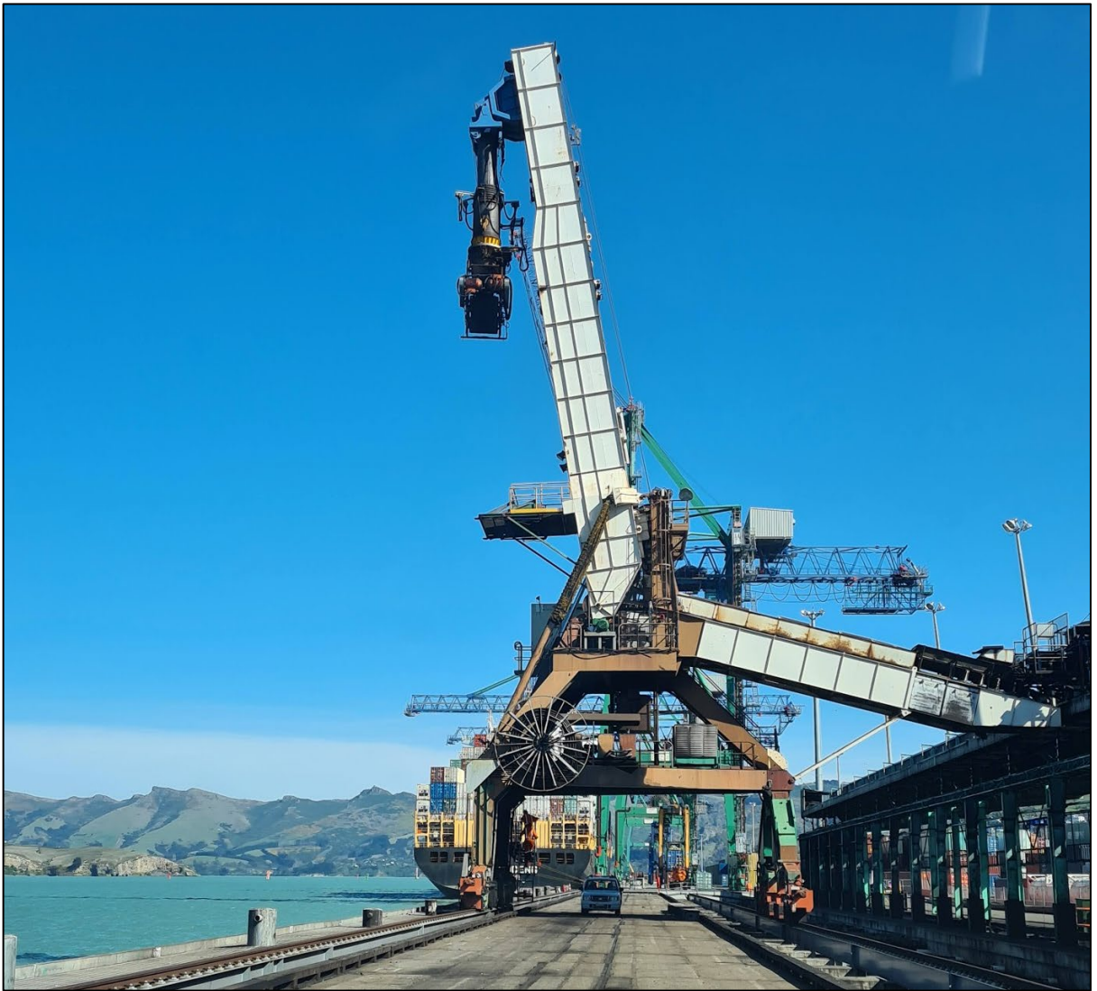
Figure 2.6: View of conveyor that can move along Cashin Quay 1 and the jet-slinger on the end that is used to load coal into a ship hold. Source: Tonkin & Taylor
