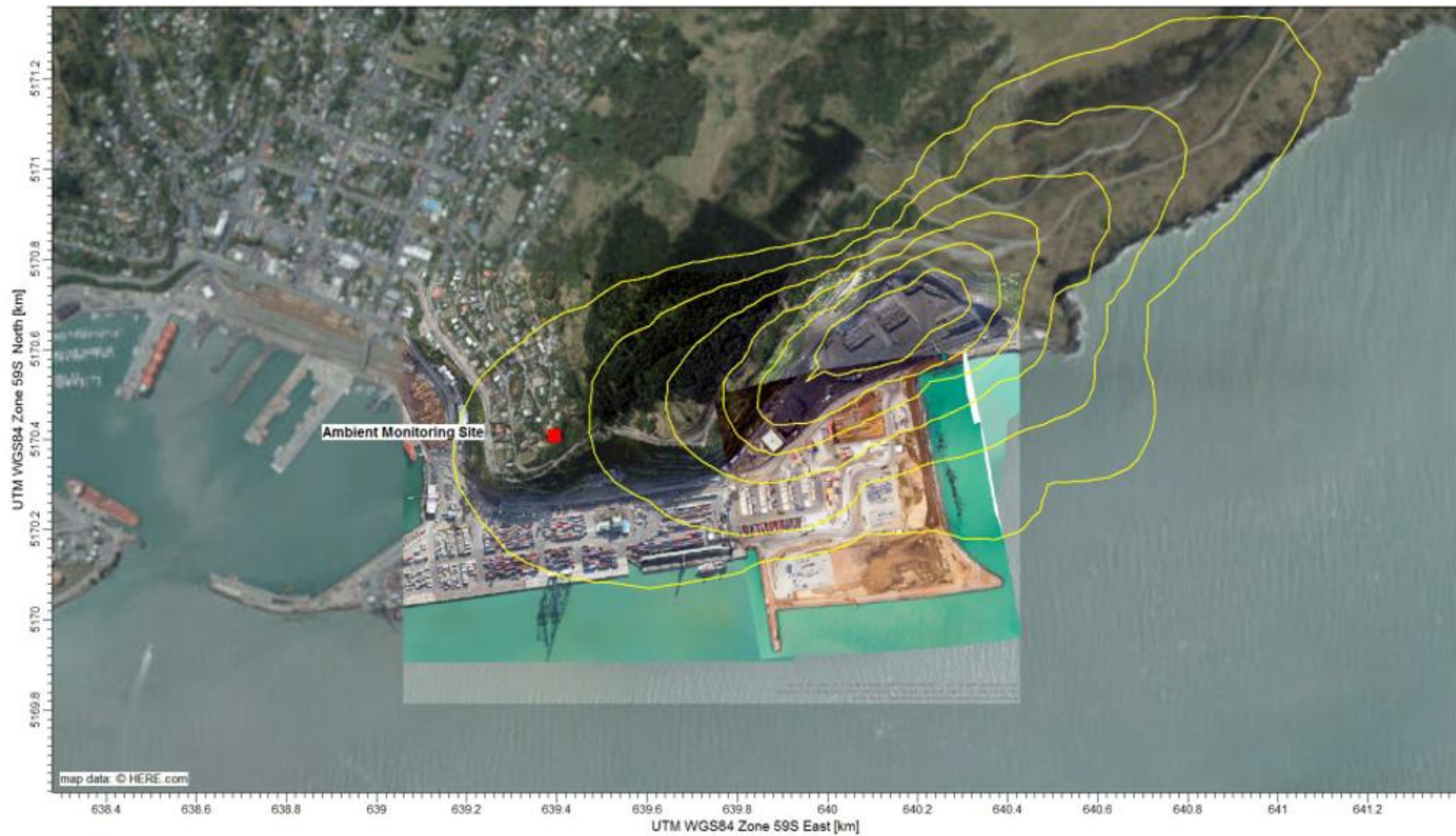
Figure 1.3: Maximum model predicted monthly dust deposition; each contour (yellow) moving in is twice the deposition rate of the outer contour and is used to depict the relative change in deposition rates with distance from the coal stockyard (T+T 2020 air quality assessment) .
