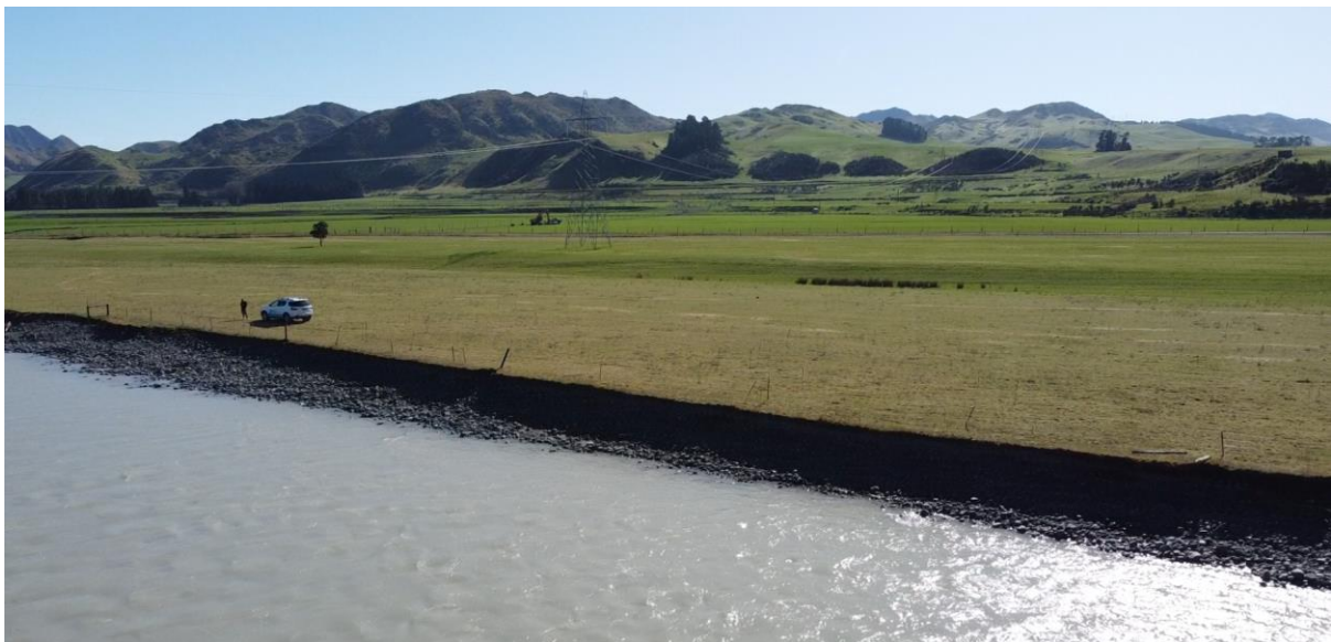
Figure 2. Drone footage of the flat flood-plain behind the location of the proposed localised ATP and the eroding bank in the foreground. A low terrace and pylons can be seen within the proposed ATP area.
