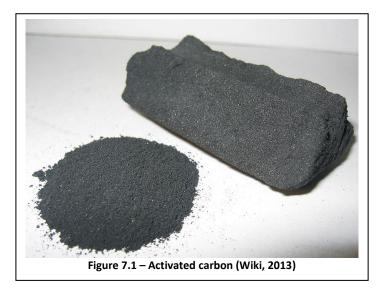
Activated carbon is carbon or charcoal that has been produced in such a way as to have many small pores that greatly increase the surface volume of the carbon, such that one gram of carbon can have as much as 2,000m<sup>2</sup> of surface area. This feature of activated carbon makes it a key component in many chemical reactions and for adsorption, where particles bind to the surface of a substance.
