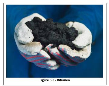
Bitumen in New Zealand is largely used for road sealing by companies such as Fulton Hogan and Isaacs. It is supplied by companies such as Z Energy and Delta Corporation, typically as a byproduct of the oil-refining process (ZE, 2013). New Zealand's bitumen market considered fairly static at approximately 165,000 tonnes per annum, with about 75% of this coming from Marsden Point oil refinery (NZLG, 2012).
