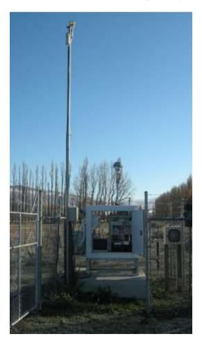
Figure I-4: An example of a temperature controlled BAM enclosure with the doors open to illustrate the BAM inside.
