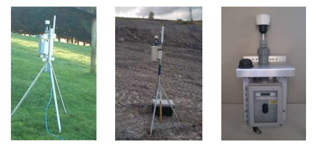
Figure I-3: Typical nephelometer installations. The unit on the left is mains powered, while the unit in the centre is battery powered. The unit on the right provides a close up.
