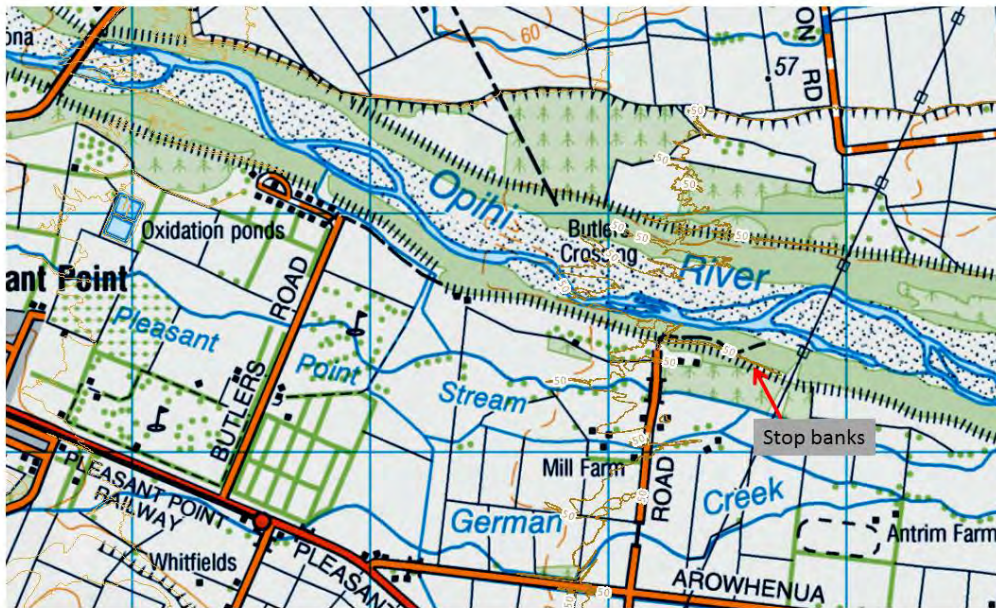
Figure A-7: 1:50,000 TopoMap of the Opihi River showing stop banking and various structures within the active surfaces
