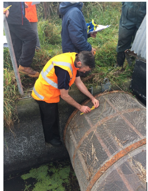
Picture 1 - Officer taking measurements of screen aperture on rotating drum
