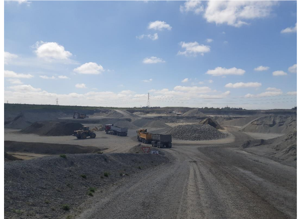
Figure 6 Pit floor. Stockpiles are not within 3m of NGL. Very minimal dust generated from loading of aggregate into trucks.
