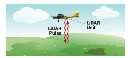
A LiDAR unit scans the ground from side to side as the plane flies because this covers a larger area. When the pulse is returned to the sensor, it contains information that can be used to distinguish features on the ground. For instance, vegetation, buildings, water and bare earth can all be determined by the characteristics of the information contained in the returning pulse. Raw LiDAR data is commonly referred to as a 'point cloud'.
