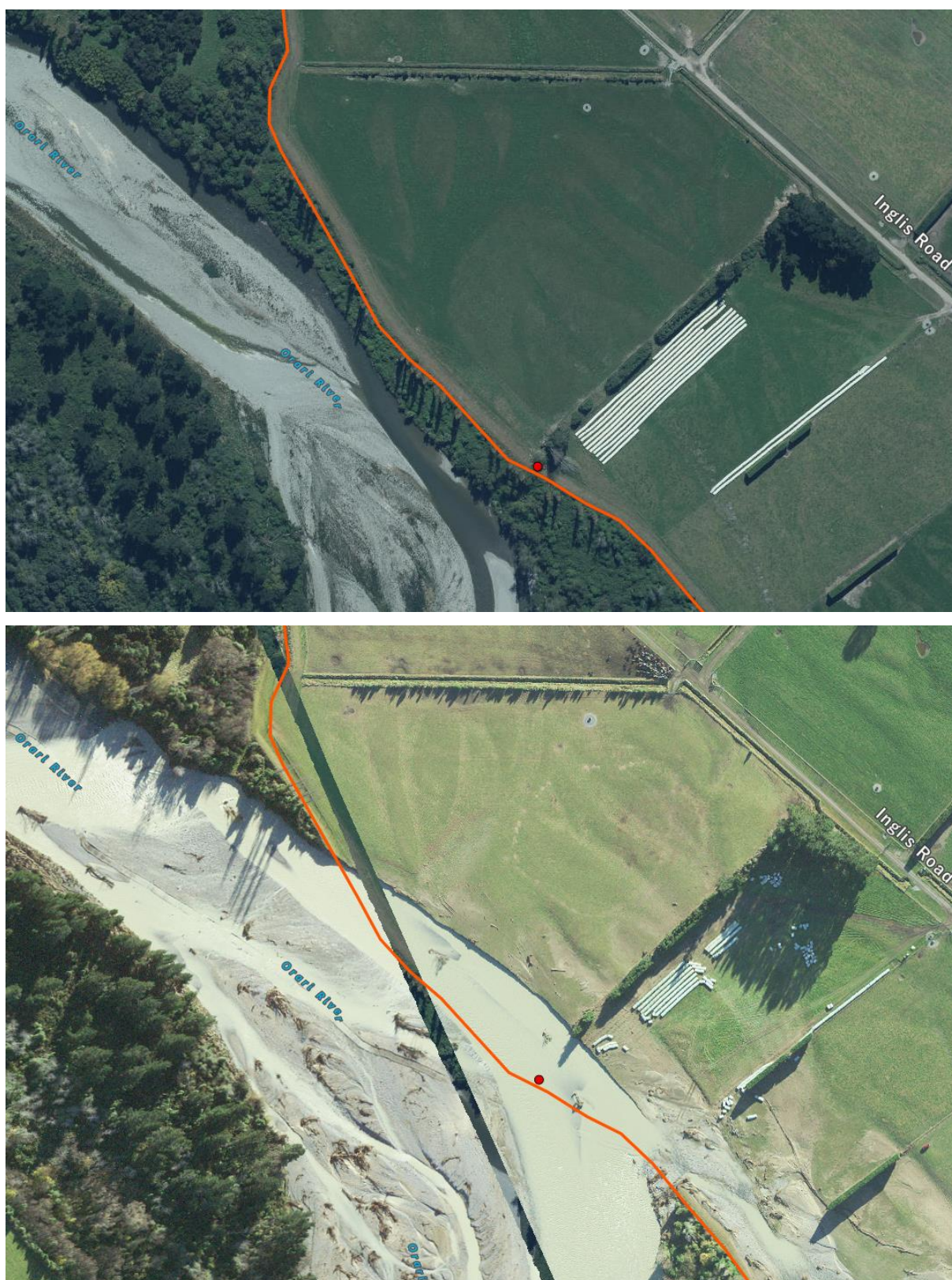
Figure A2-3: Upper Orari River. Stopbank Asset before flood (above) and loss of stopbank asset after flood (below).
