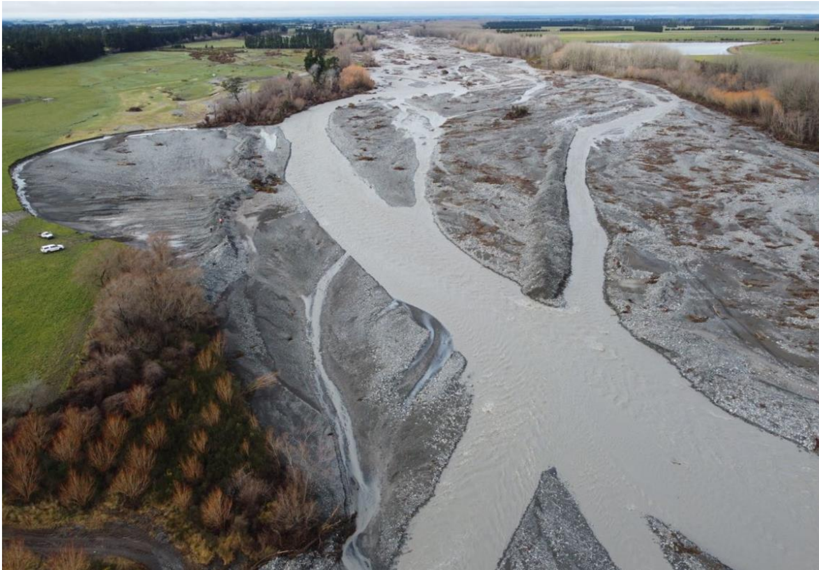
Figure A2-2: Aerial view of Ashburton River North Branch downstream of Pudding Hill Stream after flood. Note loss of tree edge protection on true left bank and some temporary bunding
