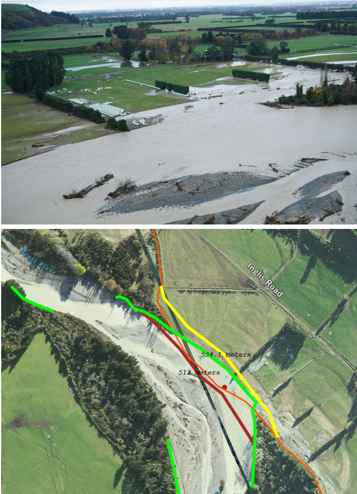
Figure A2-4: Upper Orari River. Stopbank breakthrough during flood (above) and estimate of river edge protection and stopbank asset loss (below).
